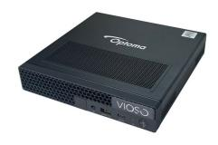
The VIOSO Nano 6 has a small footprint, about the size of a sheet of paper, but incorporates a highly powerful feature set including Intel i5 processor and NVIDIA QUADRO graphics. It is ideal for a multi-projector installation where powerful edge-blending, warping and content playback are required from one compact package.
